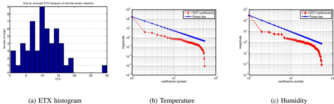
Fig. 3. ETX histogram from each node (a). Compressibility of the DCT coefficients of the temperature and humidity signal (b) (c).
